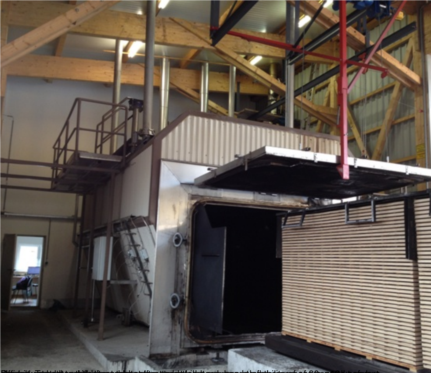
Official photo of the machine used for the tests. The machine is a large industrial oven with a capacity of 30 cubic meters.
