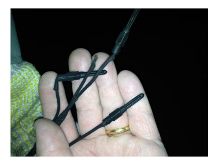
Dirty or damaged moisture measurement wires from the operational kilns. Wood moisture content is measured by measuring the elecrirn resistance of the wood and temperature of the wood. If on on these measurements fails, example becouse of not elecric connections from the measuring cable to measuring pins/nails, the moisture content of wood can not be measured properly.
