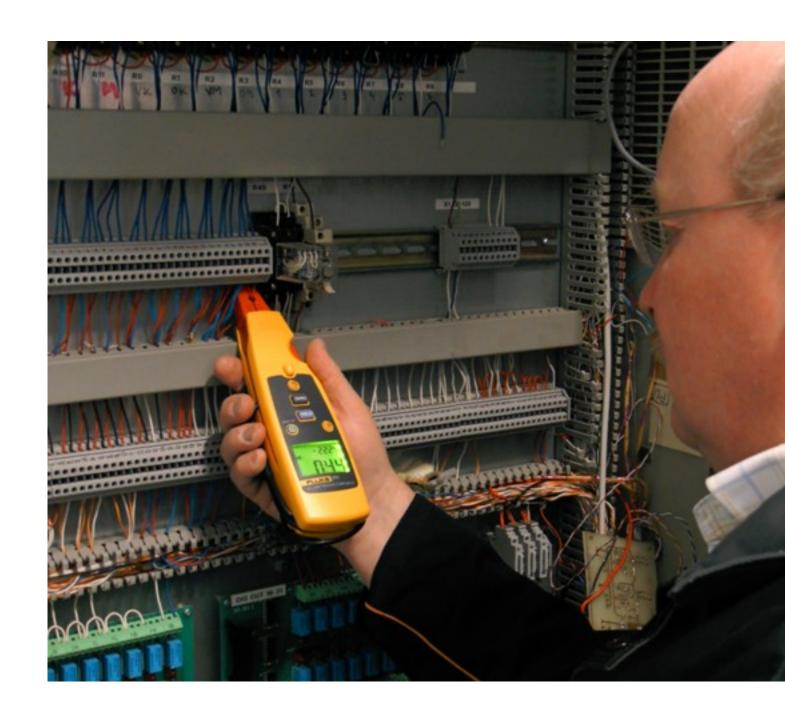
Inspection of electric calibration for valve positions.
